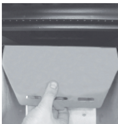
Pict. 16: Rotate the fire shield
