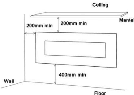
**STEP 1.** Find a safe location. Minimum clearance on each side (left, right and to ceiling) must be at least 200mm; minimum clearance from the floor must be at least 400mm; minimum clearance from the front must be at least 3 feet 3 $\frac{3}{8}$  inches (100 cm). Choose a location near an outlet so an extension cord is not required. **DO NOT** position the unit directly below a power outlet.
