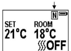
**NOTE:** It is normal for the fan heater to stop running for periods of time. This happens because the room temperature is at or above the temperature set on the remote control. The heater indicator will be turned off after 10s if you have the flame ON. The heater indicator will stay ON if you only use the heating function.
