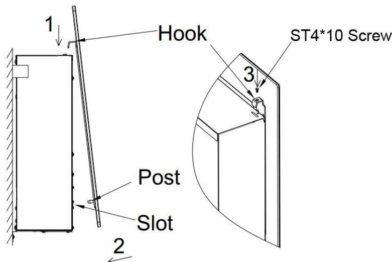
**STEP 4.** 1. Carefully set both hooks of the front glass panel into the slots at the top front edge of the firebox. 2. Press the two posts of the glass panel into the locking slots near the lower corners of the front firebox panel. **NOTE: Make sure the posts click into the slots.**
