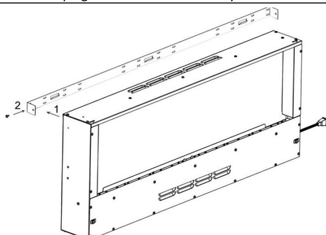
**STEP 3.** Place the fireplace in front of / on the bracket (see 1) and screw the fireplace to the bracket with the ST4x10 screws on left and right side (see 2).
