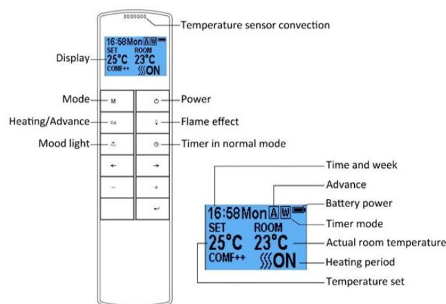
**NOTE:** This is a thermostatic remote control. The remote should be in the same room as fireplace and placed on a flat surface. It must be placed away from the heater so the hot air will not blow on it and affect thermostatic reading.
